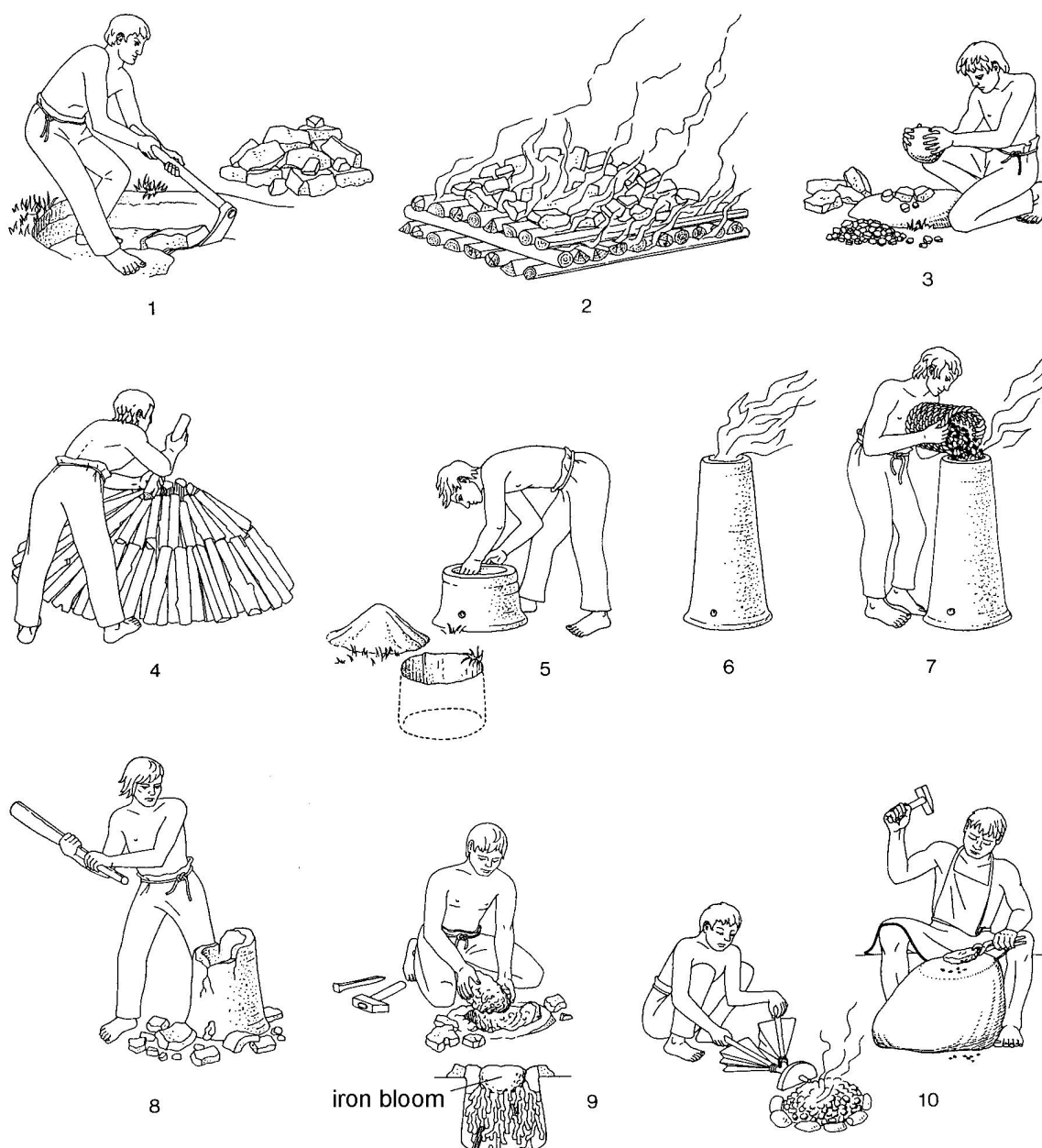
Fig. 43. Production stages during the processing of iron ores.
